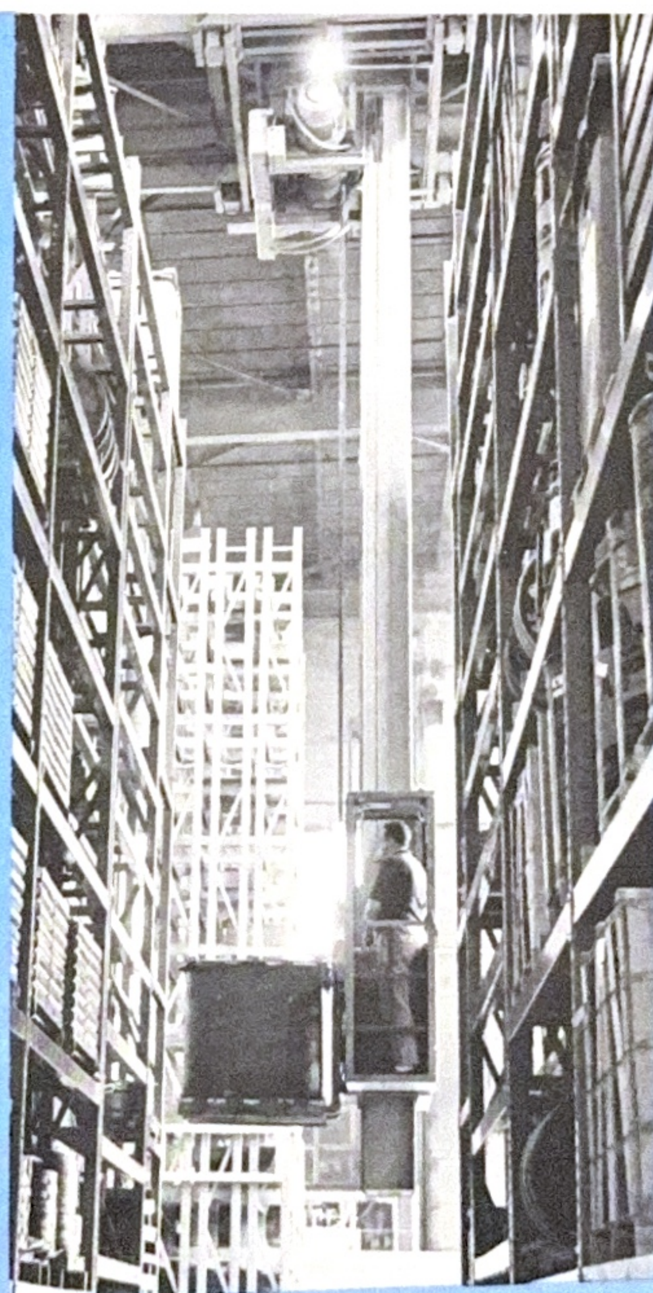
MOVED VERTICALLY and horizontally by operator Norbert Dvorsky, the stacker crane (left) slides out parts and material containers for delivery to production areas. In the new storage area, lift truck operator Philip Raimondo has plenty of room for movement.
