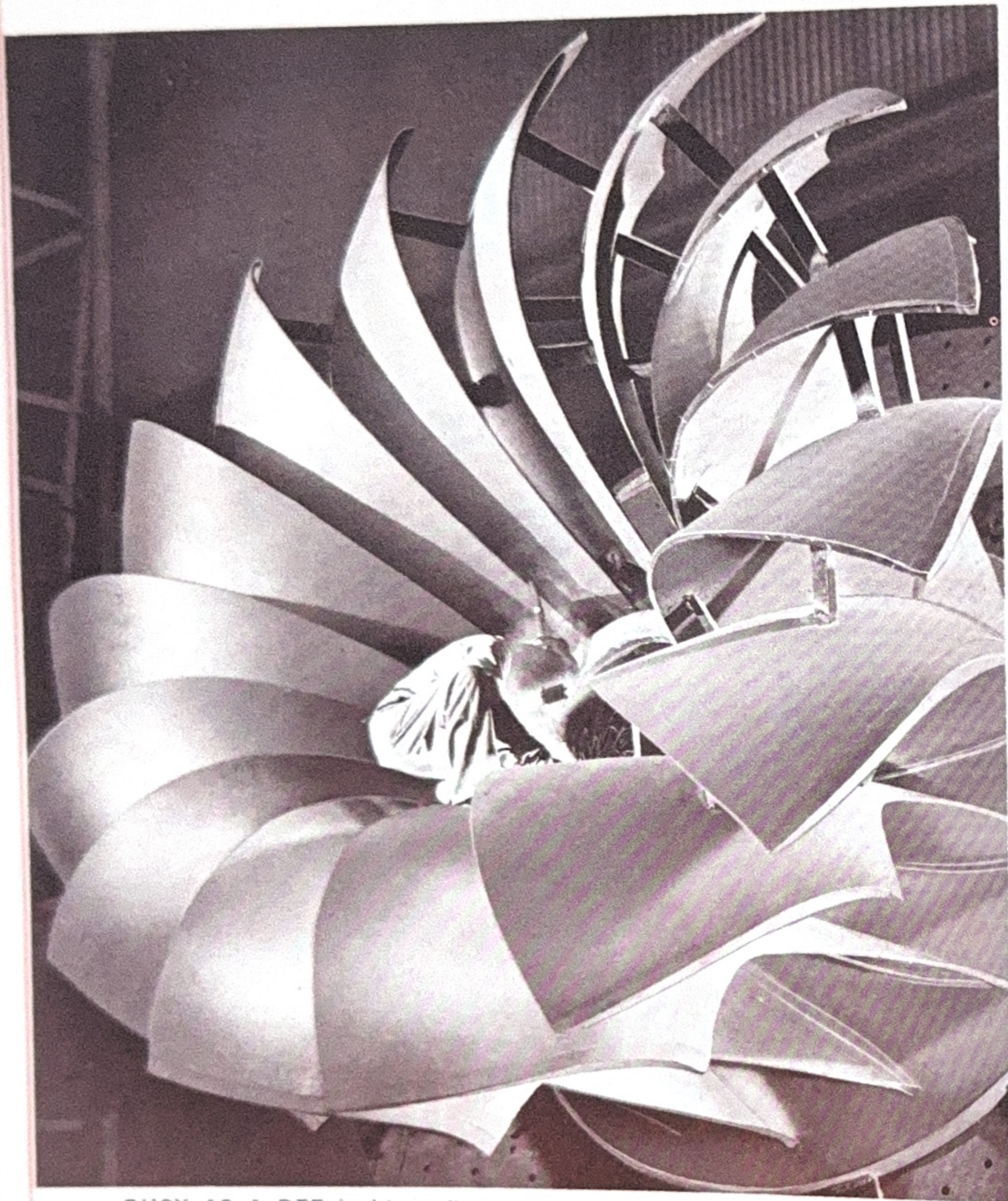
BUSY AS A BEE inside a flower is this welder at the York Plant. Actually, these steel petals comprise a partially completed runner for a hydraulic turbine that will be installed in a hydro-electric plant in Liberia, Africa.
