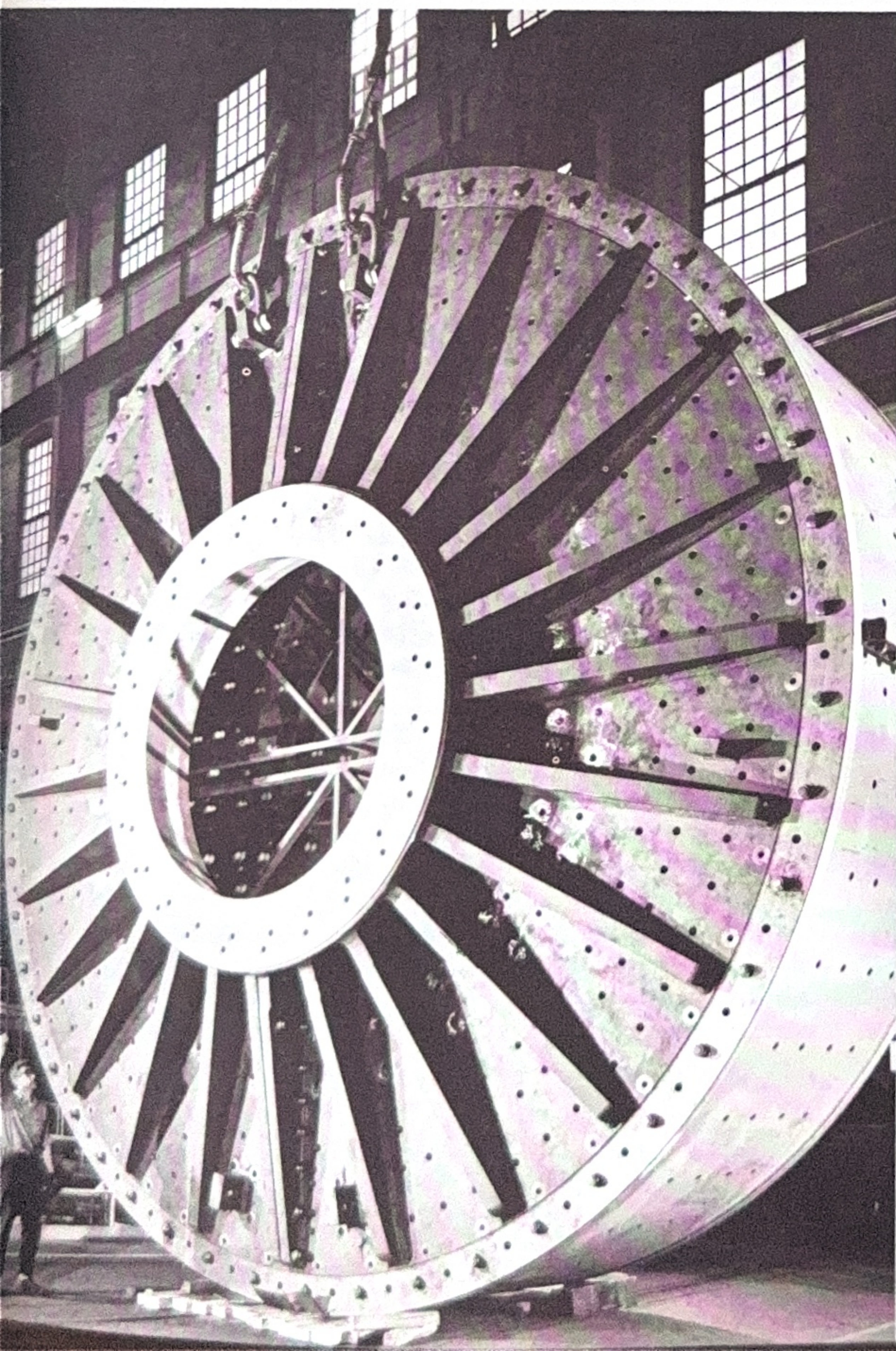
THE HITCHER is dwarfed by this huge grinding mill, said to be the largest in the world. The mill is part of a $3½ million order for the Hanna Mining Co. We are manufacturing 12 autogenous grinding mills, each of which weighs over 250 tons and is 28 feet high.
