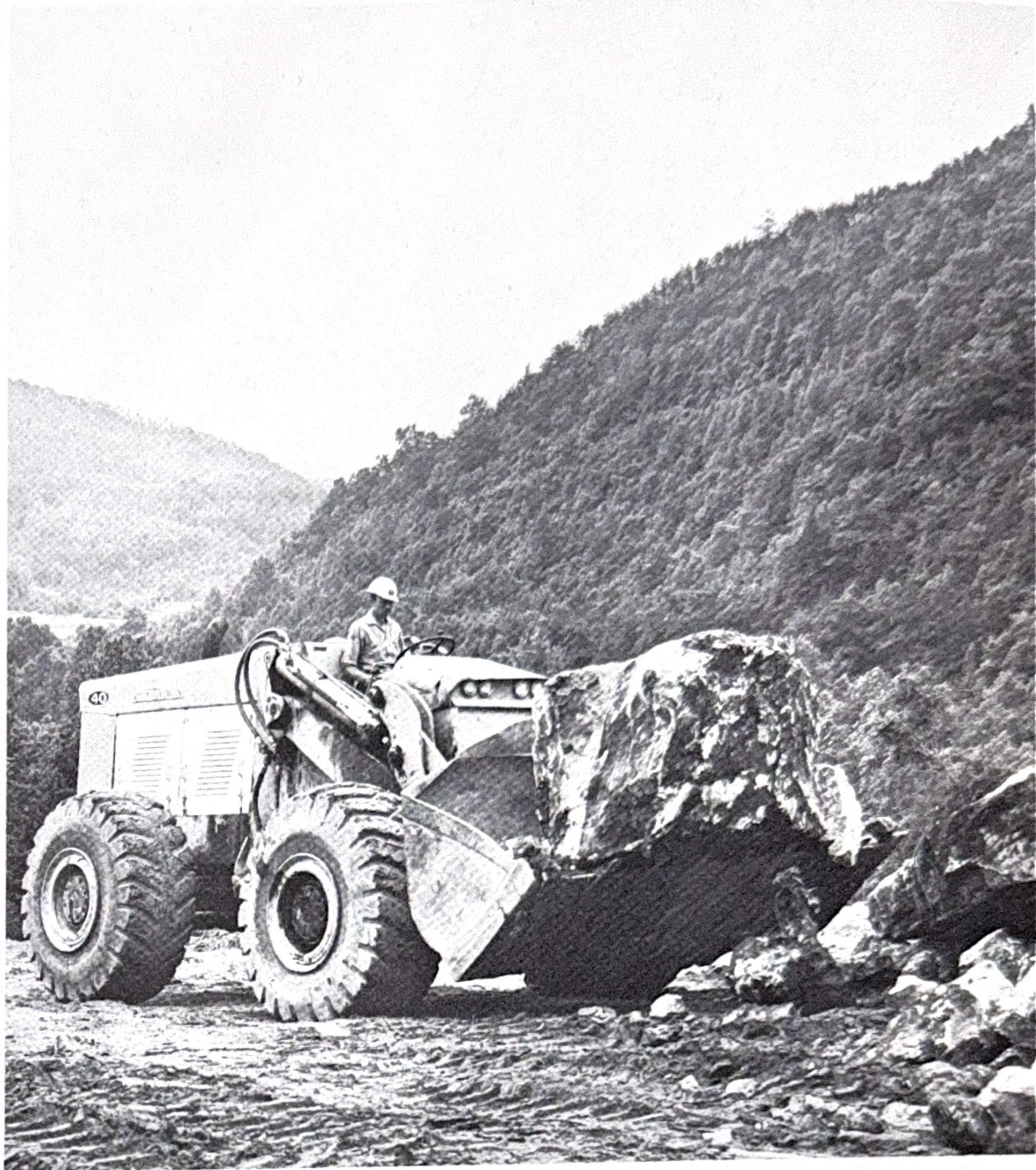
Twenty-three tons of rugged power for construction machinery projects is available in the Deere-made TL-40 tractor loader, one of a number of new A-C models.
