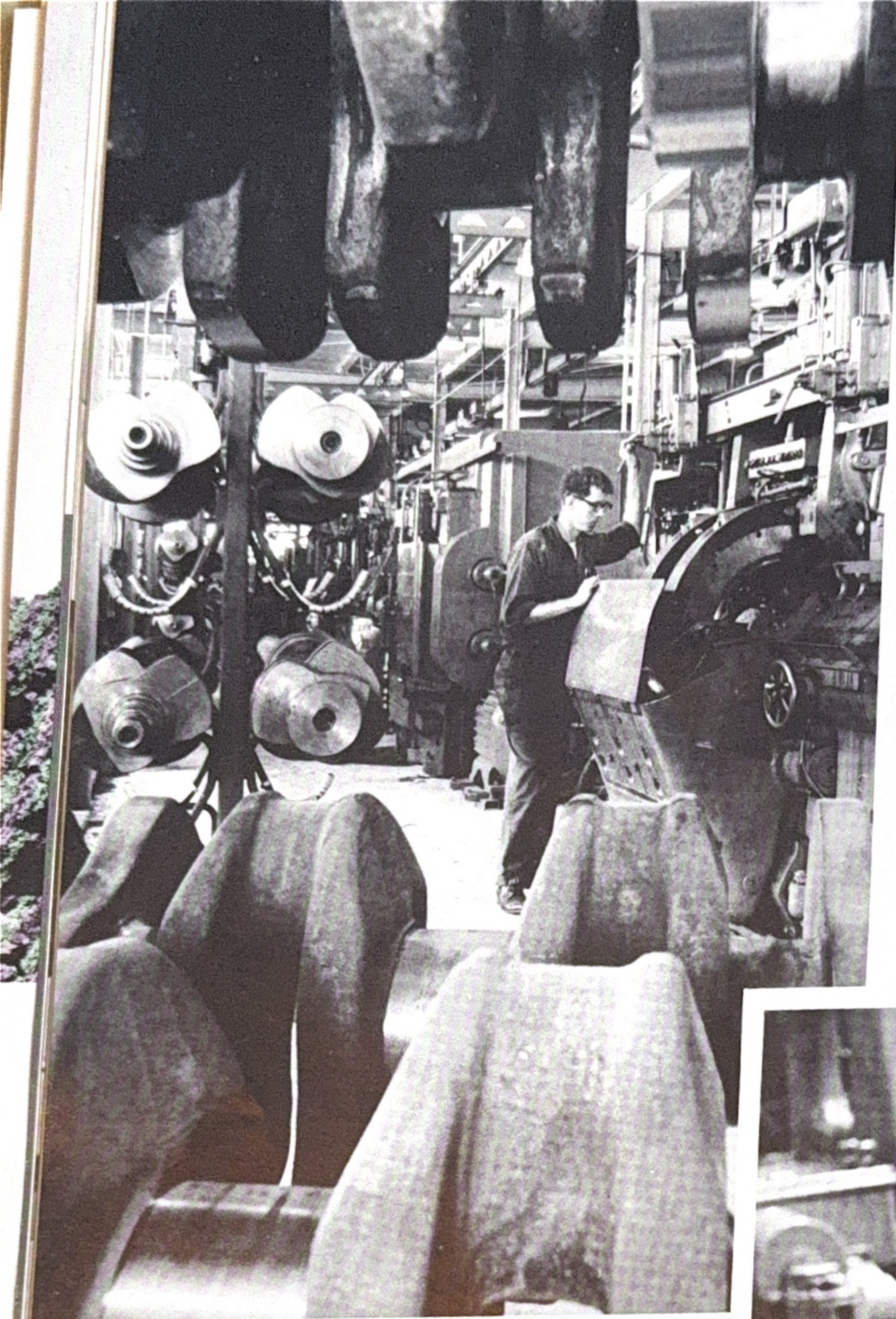
An "iron curtain" effect is created by these crankshafts. They frame the finish grinding operation at the engine crankshaft production line, Harvey Engine Plant. The employee is James Mangrum.
