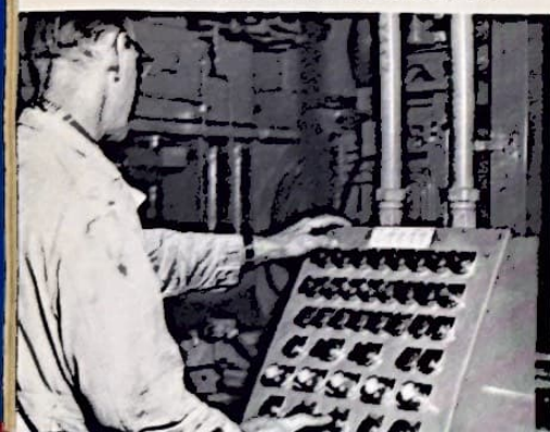
To set up proper machine sequence in milling of cylinder blocks, Maurice Howard presses a series of buttons on the control panel.
