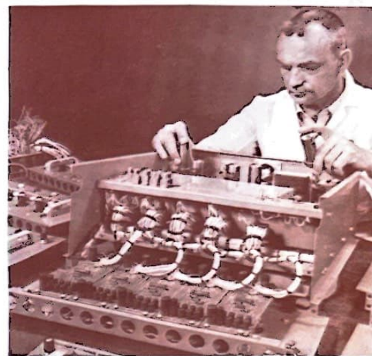
This CSC-designed control system operates valves, pumps and controllers for a petroleum refining miniature pilot plant.
