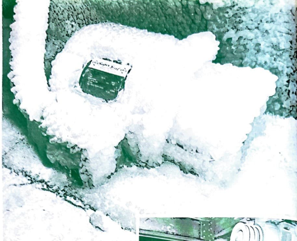
An ability to take the most adverse conditions in stride has become the mark of Allis-Chalmers motors. Thickly coated with ice is a Super-Seal motor undergoing a torture test.
