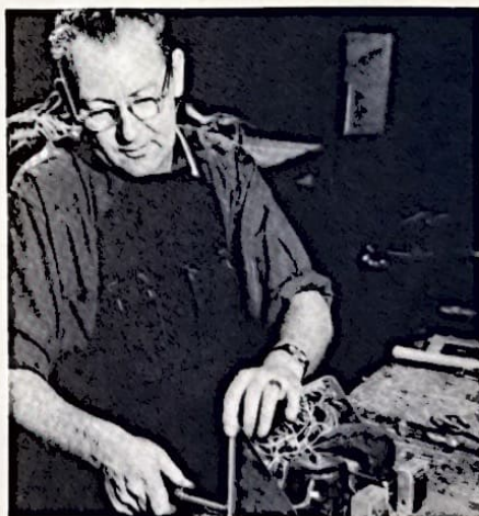
Assembling a static regulator of the type used on the sets is Glen Phillips, Hawley Shop, West Allis Works. The sets are nearly identical to those we are making commercially available day after day.
