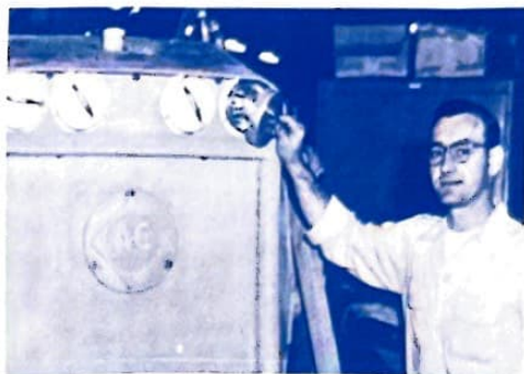
A device resembling a cookie-cutter gained Marvin Slosser, Deerfield Works Assembly department, $150. It is placed over lamps prior to spraying, eliminating masking.
