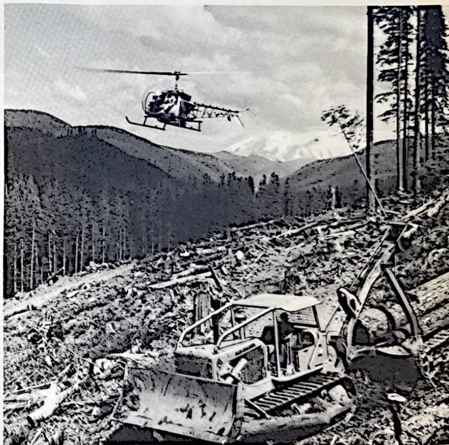
HD-21 crawler tractor, built at Springfield Works, is shown skidding a load of logs out of a Washington forest amid majestic scenery. Helicopter in scene is engaged in aerial seeding of a tree farm, simultaneously with the logging operation.
