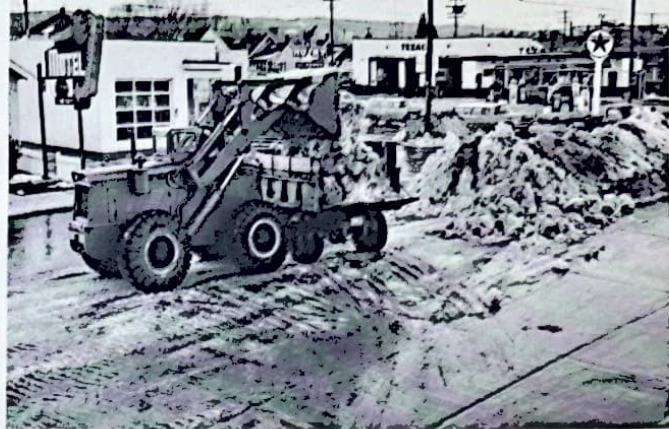
TL-20, largest unit made at Deerfield Works, typifies all-around ability of rubber tired wheel loader in municipal service. These units remove snow in winter, also work in park and street service.
