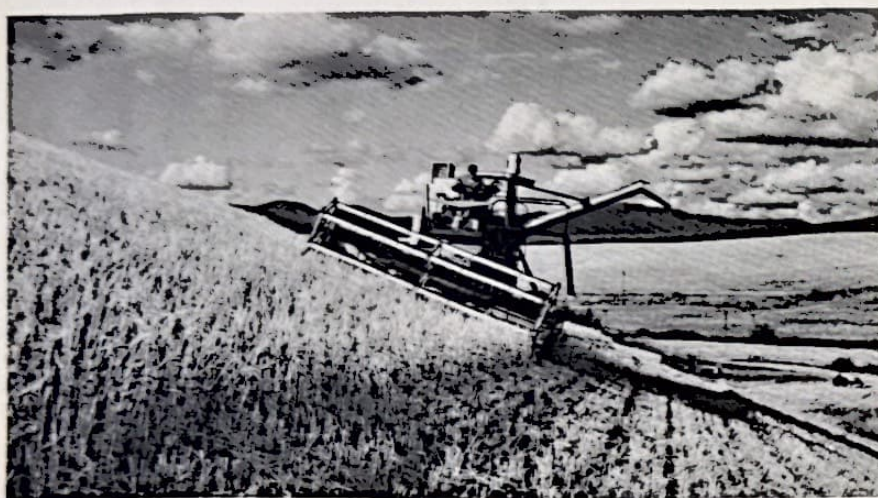
The "hillside" Gleaner-Baldwin combine, built at Independence Works, is one of the new harvesting machines developed and tested by A-C in 1959 for sale this year. The unit was subjected to extensive field testing, with outstanding performance results.
