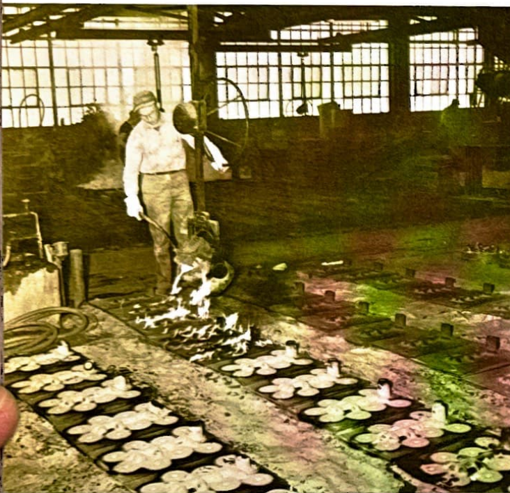
Being poured in the LaCrosse Works foundry, these castings may be used in the plant's farm implement line or may be destined for one of several other A-C plants which utilize LaCrosse castings in their products.
