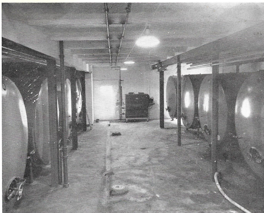
The new glass-lined fermenting tanks that have been installed as part of the Oshkosh Brewing Co.'s continuing modernization program.
