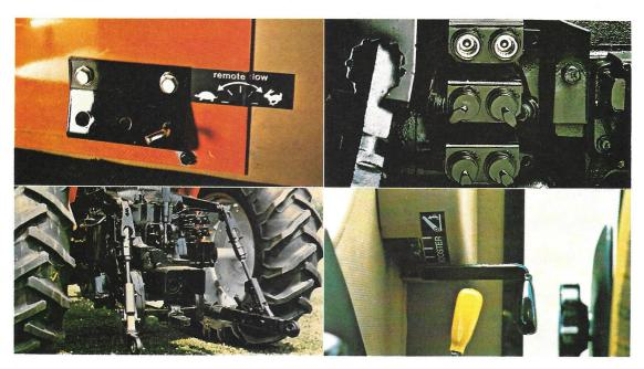
Pressure-compensated flow controls (one standard, two optional) permit adjusting flow rate for each remote valve independently, increasing remote hydraulic versatility. Flow is controlled even when two or more valves are operated simultaneously.
