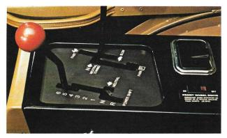
Shock-free operation. Forget about abrupt or lurching speed changes. Shifting is smooth because torque is always maintained. Of the two clutches used in any speed, one always remains engaged while the other is
