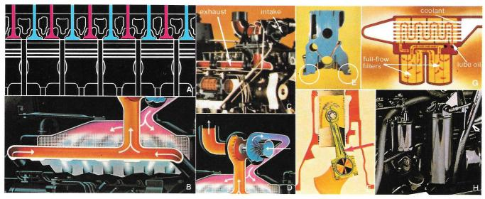
A. Alternating intake and exhaust valves. In the 670 Series engines, valves alternate the full length of the block to reduce hot spots and increase valve life. Rotators on intake valves cool down areas where heat might flare up.
