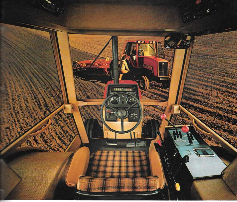
Step up to comfort and convenience through either of two doors—with the help of non-skid steps and easy-to-reach grab handles—the best cab entry story ever. A compressed gas cylinder in the door makes opening easier, and a light comes on in the cab just like in your car. The outside door latches are located at the bottom of the door where they are easy to reach (shown above).
