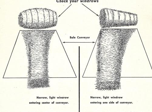
Make double windrows  $3\frac{1}{2}$  to  $4\frac{1}{2}$  feet overall width for shapely rolled bales.
