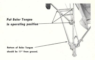
Tractor Wheels set too wide or Baler Tongue in transport position will cause tractor to run on windrow
